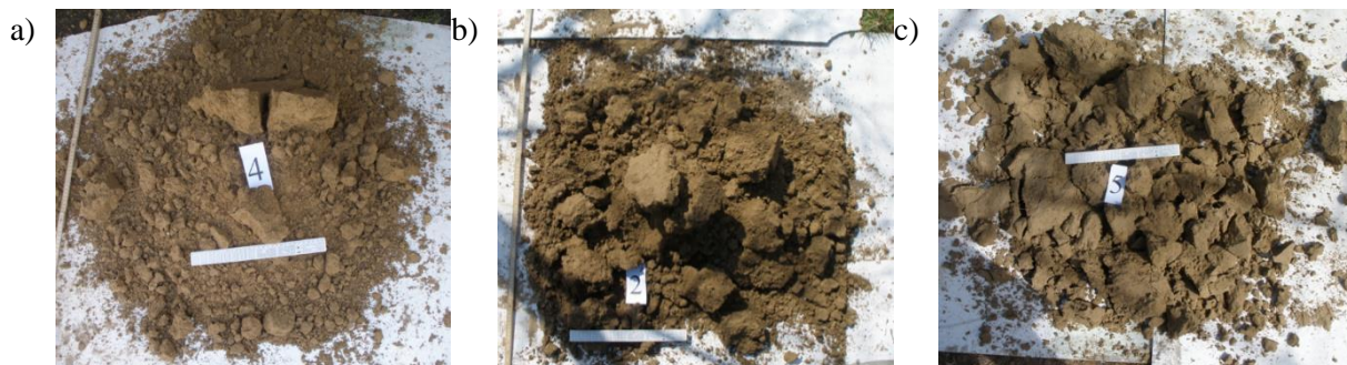
Fig. 1. Soil comminution in individual experiments after falling from a height of h = 1.1 m: a – light sandy soil; b – medium sandy soil; c – light loamy soil
